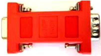
**Figura 3.3.31 Conector lookback adapter para comprobar retorno en puerto serial**
